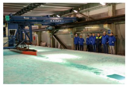
The testing, completed at a large indoor testing basin at Aker Arctic in Finland, provides a proven and effective means of ensuring Seabourn Venture's hull design will perform as intended in the ice conditions it may encounter. A ship rated to PC-6 Polar Class standards is capable of summer & autumn operation in ice conditions in <u>Antarctica</u>, the Arctic, and other exotic destinations around the world.
